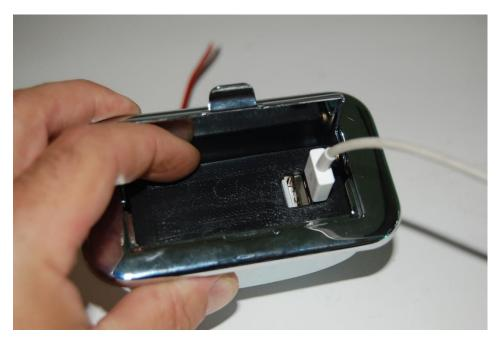
With the appropriate size crosshead screwdriver (a battery drill works best) drive the self tapping screws into the plastic housing through the 4 holes. They just need to be snug, no impact required.
