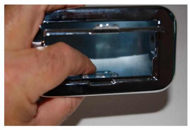
2 Drill a 1/4" or 6mm hole in the bottom face of the box.
