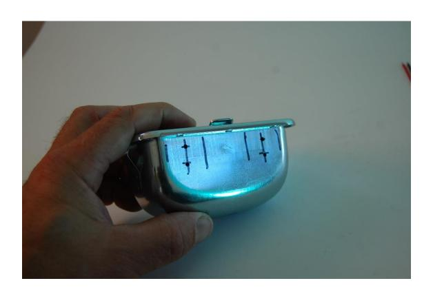
4 Poke the wire through the grommet and hold the ashtray centrally against the stubber side of the box. The stubber acts to locate it from side to side. The top face of the recess in the front of the USB housing should sit against the stubber to give the correct height.
