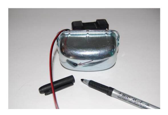
Mark two vertical lines with a pencil on the outside of the box,
